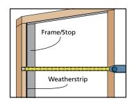
allow 1/8" clearance on the head jamb and 1/2" between the bottom of the slab and the top of the threshold.
