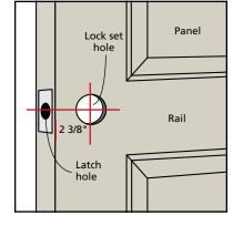
the lock set is usually centered in the rail (horizontal member) across the center of the slab or 35" from the bottom of the slab (not the sweep). Lock set holes should be either 2 3/8" or 2 3/4" on center from the edge, depending on the latch.
